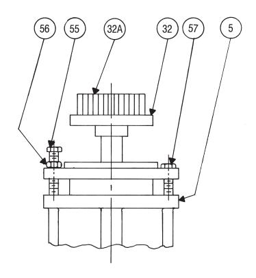
b. Check angular alignment with a micrometer or caliper. Measure from the outside of the one flange to the outside of the other at intervals around the periphery of the Coupling. Determine the maximum and minimum dimensions. DO NOT rotate the Coupling. The difference between the maximum and minimum must not exceed .O10". If a correction is necessary, be sure to recheck the parallel alignment.
